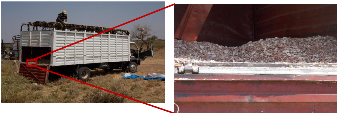
Figure 2: Truck floor modified with saw dust
