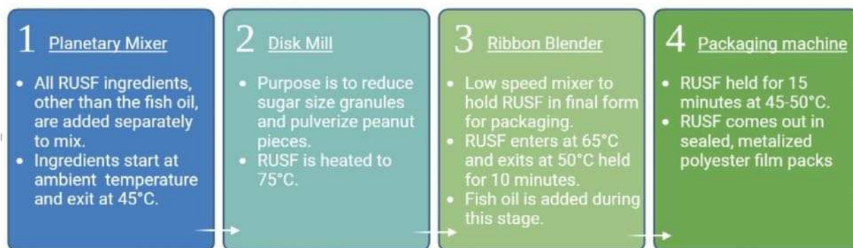
Figure 1: Maternal ready-to-use supplementary food manufacturing process
