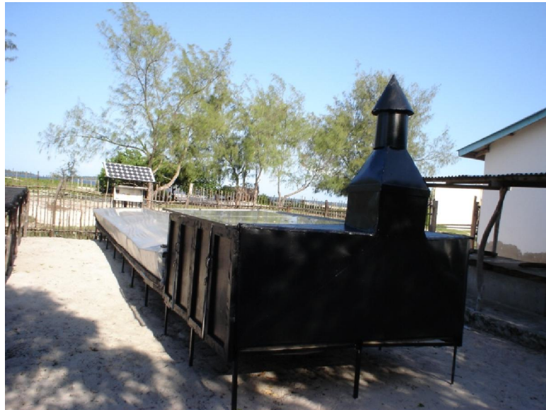
Figure 2: The solar tunnel dryer in Gazi, South coast of Kenya
