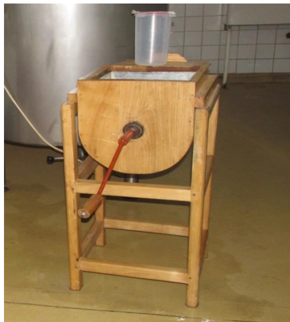
Figure 1: Hand-operated churner made from wood and lined with aluminum sheet. It consists of a shaft fitted with baffles. A woman performed the churning when seated and rotated the shaft through the crank to allow the baffles to cause a vigorous mixing that results in coagulation of the butter and separation from the rest of the fermented milk. The churner shown has a capacity of 15 liters, but higher or lower capacity units can be made
