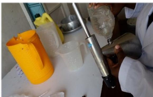
Figure 2:Filling alcohol gun with alcohol
