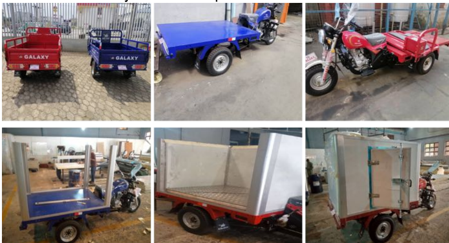
Figure 2: Construction of insulated chamber
