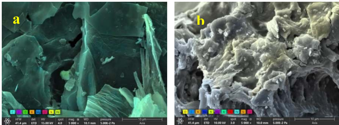
Figure 1: Detail view of (a) BC and (b) MBC pore structure under the scanning electron microscope (SEM) indicating pores filled with digestate after incubation for 21 days
